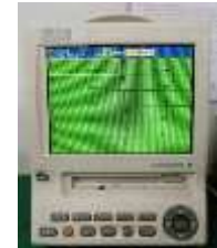
Multi-channel Temperature Detector
